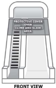
FIG. 8 Protective Cover Over Slide and Climb Area
