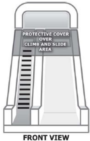
FIG. 8 Protective Cover Over Slide and Climb Areas
