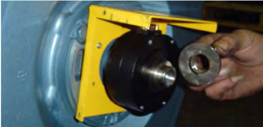
Photo 1 - Apply adapting socket to the end of the motor shaft. (Contact factory for availability of socket.)
