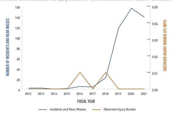
Figure B2: Injuries and Fatalities for Uninsured Boilers and Pressure Vessels (2012 - 2021)
