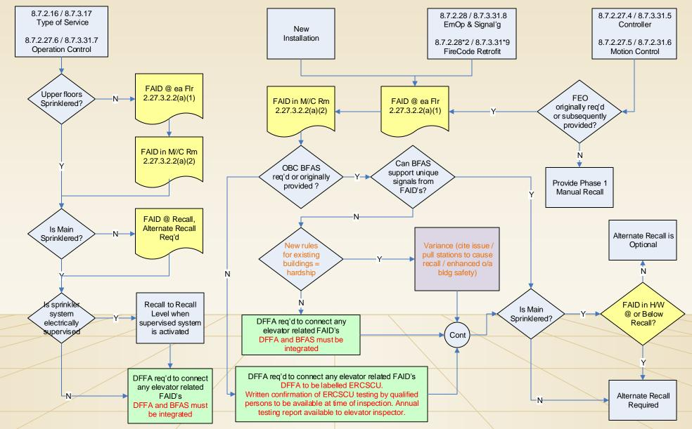
OBC -Ontario Building Code FAID – Fire Alarm Initiating Device BFAS – building fire alarm system DFFA – Dedicated function fire alarm FAID – Fire Alarm Initiating Device ERCSCU – Elevator Recall Control and Supervisory Control Unit
